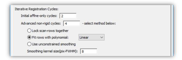
The first type is to correct the scan-distortion using only affine transformation. This type of transformation is a 'linear non-rigid transformation'. Linear, because any straight line feature before correction will be preserved as a straight line afterwards, and non-rigid because different pixels can move by different amounts in x and y. Using this type of iteration the user can correct for image shear, scale, and (small) rotations.
