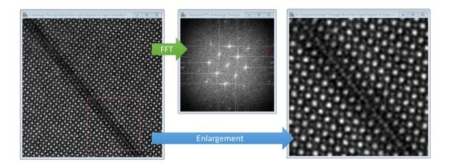
After processing the (331) spot is visible (approx. 0.9Å resolution), and the detail in the interface become clear. The recovered resolution is likely slightly poorer than had the image been recorded under optimal sampling conditions, but it is an improvement on the raw data.
