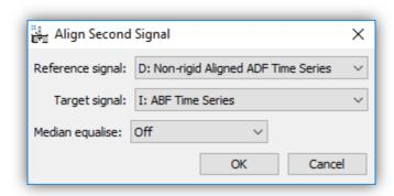
Here for example the diagnosis from the registration of an ADF series is copied to an ABF series. After pressing OK, both the new aligned signal will be displayed as well the average of the new series.
