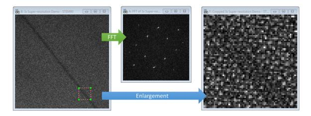
The FFT shows spots are visible right out to the Nyquist limit, and the highest observable spot is the (220) spacing (approx.. 1.38Å. A 64x64 pixel ROI is enlarged on the far right – again, not how the sampling is too low. Ordinarily this would be a poor choice of setting to record the image; we would usually increase the number of pixels or reduce the field of view (increase magnification). However, both these options would increase the total electron-dose over the sample.
